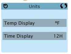
Press "Temp Display" to change the temperature between Fahrenheit and Celsius. Press "Time Display" to change the clock between 12 hr and 24 hr display.
