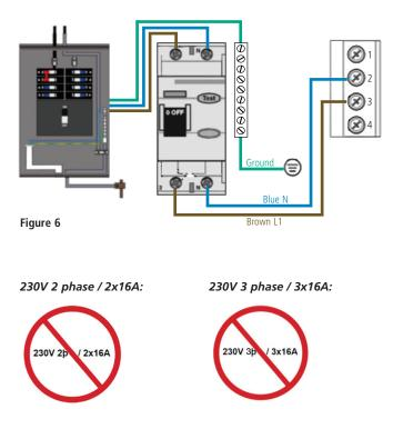
\* Must be sized to spa specification. Spa rated maximum ampacity cannot exceed the service maximum ampacity. This does not represent an option to the Installer.
