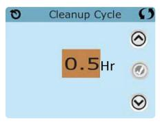
Note: Cleanup cycles do not apply to systems set for 24hr circulation pump mode as the circulation pump performs as the heat and filter pump to provide constant filtration.
