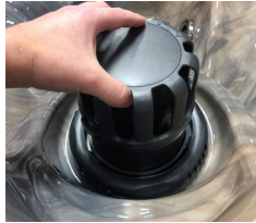
Pull Up to Remove Floater Assembly
