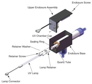
Figure 2: Spa Solar Eclipse Exploded View
