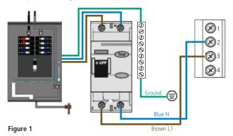
**Optional 1:** Dual Service, TN and TT Electrical Systems (2x16 Amp). 5 Wires (2 Lines + 2 Neutrals + 1 Protective Earth)\*. Protective Earth wire (Green/Yellow) must be connected to system ground terminal as marked. The heater runs on service line L1. All equipment (pumps, etc.) runs on service line L2.
