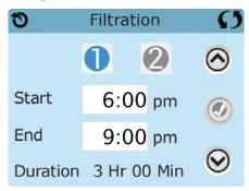
Press "1" to view Filter 1. Press "2" once to view Filter 2. Press "2" again to turn Filter 2 ON or OFF. When Filter Cycle 2 is ON, it can be adjusted in the same manner as Filter Cycle 1.
