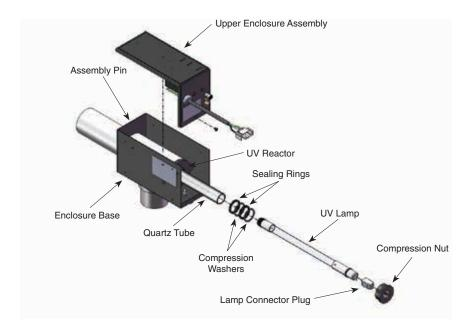
Figure 2: Mast3rPur System Exploded View
