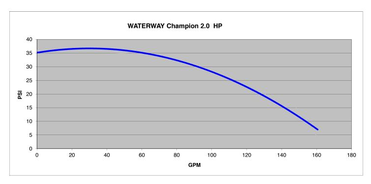
Pump curve supplied for installers where recommended pump is used.
