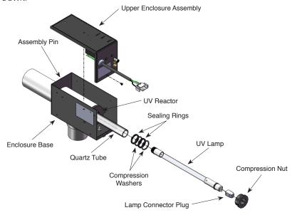
Figure 2: Mast3rPur System Exploded View
